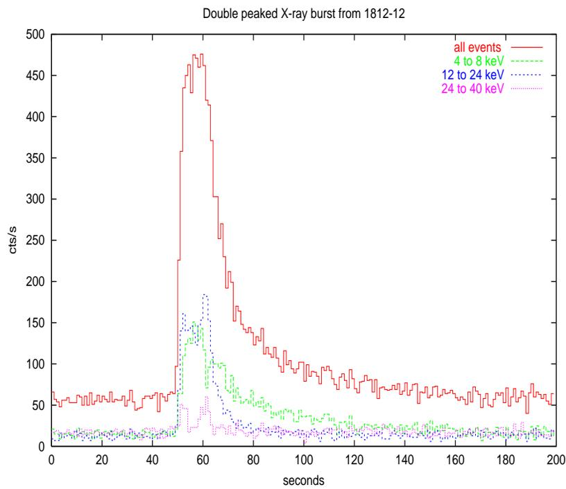
**Fig. 4** X-ray burst from 1812–12. Note double peak at highest energies.
