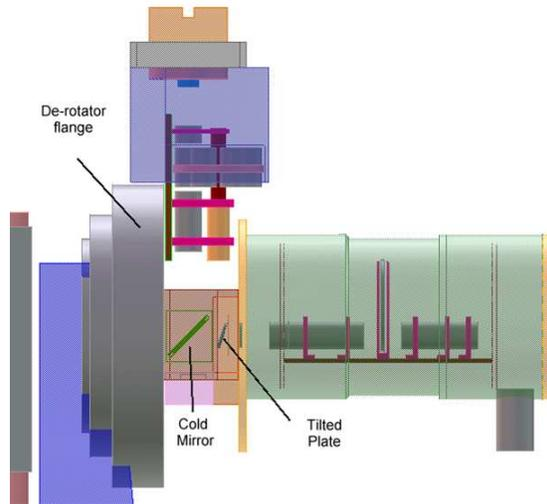
Fig. 5 The Nasmyth focus is bent 90 degrees to accommodate ROSS.
