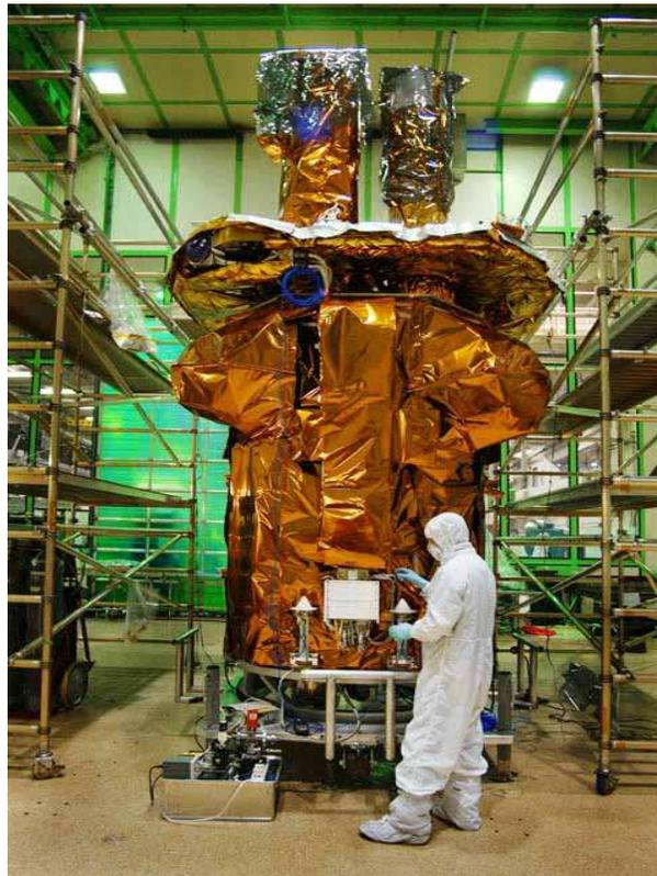
Fig. 6 The Swift satellite in the clean room at the GSFC, with the XTR and UVOT telescopes already mounted on the satellite.
