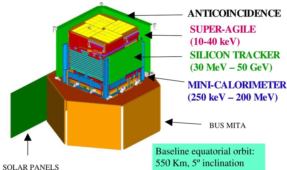
**Fig. 1** The AGILE instrument size is  $\sim 63 \times 63 \times 58.5 \text{ cm}^3$  for a total payload weight of  $\sim 130 \text{ kg}$ .
