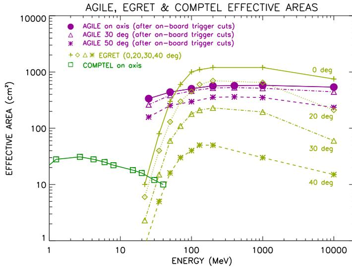
**Fig. 4** AGILE effective area as a function of energy for several off-axis angles.
