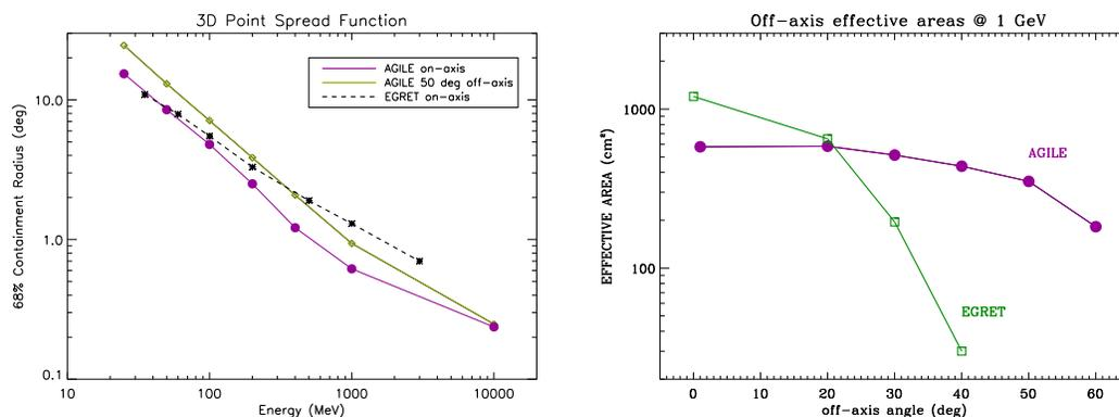
**Fig. 3** Left panel: AGILE 3-D PSF. Right panel: AGILE effective area as a function of the off-axis angle.
