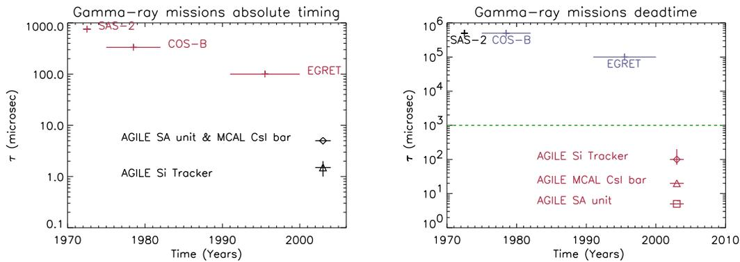
**Fig. 5** AGILE excellent timing capability.
