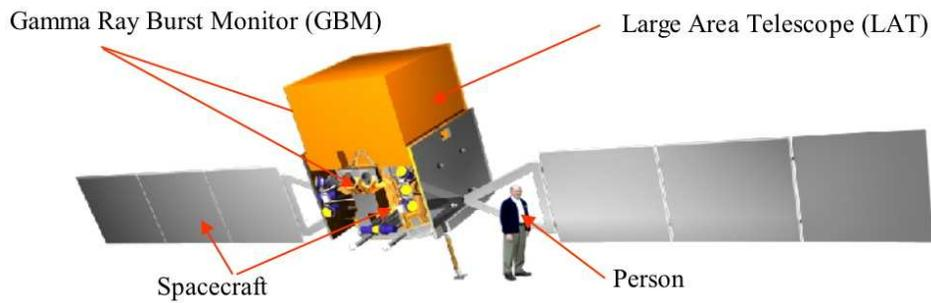
**Fig. 1** The GLAST payload.
