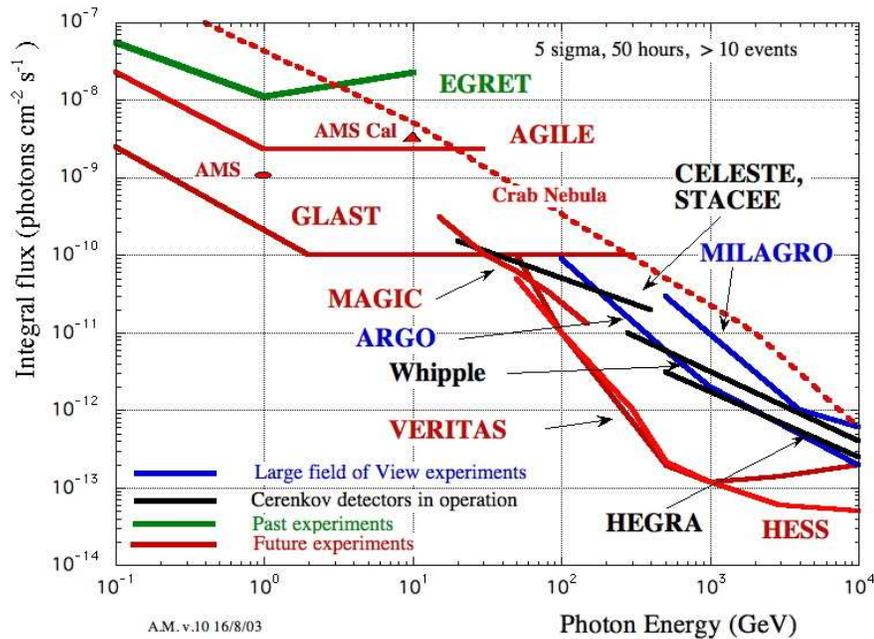
**Fig. 6** Sensitivity of present and future detectors in the gamma-ray astrophysics.
