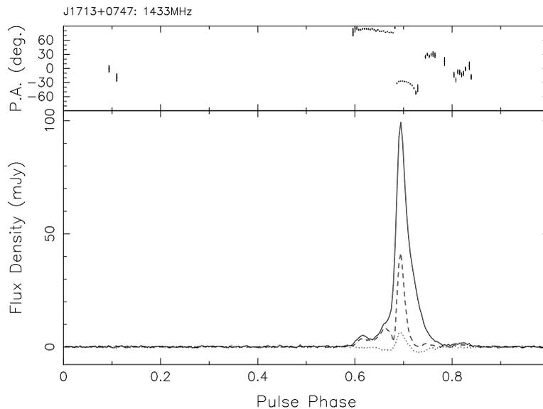
**Fig. 2** Polarisation of the mean pulse profile for the MSP PSR J1713+0747 at 1433 MHz recorded with the prototype digital filterbank system at Parkes. In the lower part of the figure, the solid line is total intensity (Stokes  $I$ ), the dashed line is linearly polarised intensity ( $L = (Q^2 + U^2)^{1/2}$ ) and the dotted line is circularly polarised intensity (Stokes  $V$ ). The upper part shows the position angle of the linearly polarised component.
