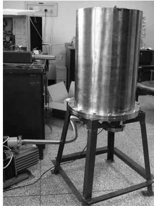
**Fig. 3** This picture shows the dewar and the rotatory pump.
