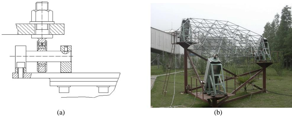
**Fig. 3** Structure of self-adaptive connector and the picture of 1:3 scale model.
