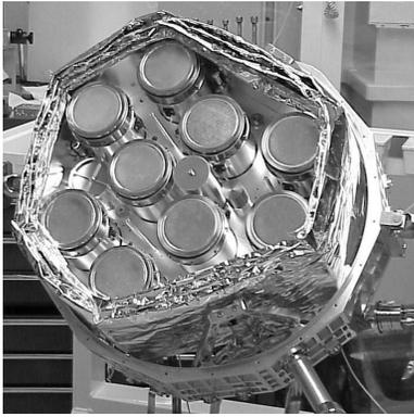
**Fig. 1** The RHESSI spectrometer array showing the array of nine large Ge detectors. Near the center of the array is a large LN<sub>2</sub> tank used for pre-flight testing. Just to the right of the LN<sub>2</sub> tank is the small Be scattering block used for polarization studies.
