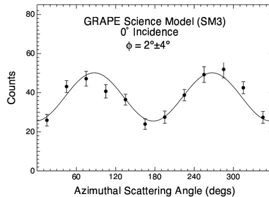
**Fig. 4** A measured result from laboratory tests of a single GRAPE module. The measured polarization level of  $\sim 56\%$  is consistent with that expected from the scattered beam of 662 keV photons used for the test.
