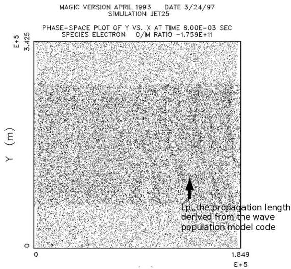
**Fig. 4** This figure shows the PIC simulation of a jet-ambient-medium for the same parameters associated with Figure X, but with the propagation length for the wave population code marked. As can be seen, the propagation length,  $L_p$ , is coincident with the position in the plasma where the plasma waves have developed significantly.
