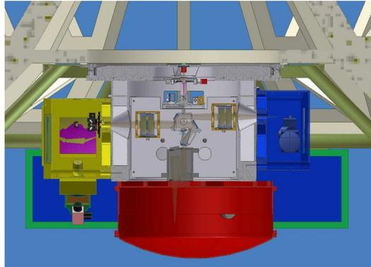
**Fig. 2** X-shooter general layout. The backbone, shown attached to the Cassegrain focus of the VLT, contains the pre-slit optics pre-processing and dispatching the light into the UV (left), the VIS (right) and the IR (bottom) arms.
