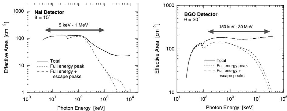
**Fig. 2** The effective areas of GBM NaI (Tl) (left) and BGO (right) as a function of energy.
