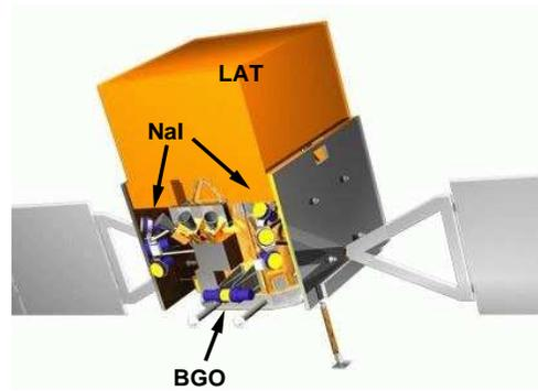
**Fig. 1** A schematic view of the main body of the GLAST satellite with the detectors of the Gamma-Ray burst monitor (GBM) emphasized. The 12 NaI-detectors are mounted in 4 groups on the outside of the satellite (two groups are visible in this view). Each group is equipped with 3 NaI-detectors viewing in different directions. The two BGO-detectors are mounted on opposite sides of the satellite (one is visible in this view). *Original image from SpectrumAstro.*
