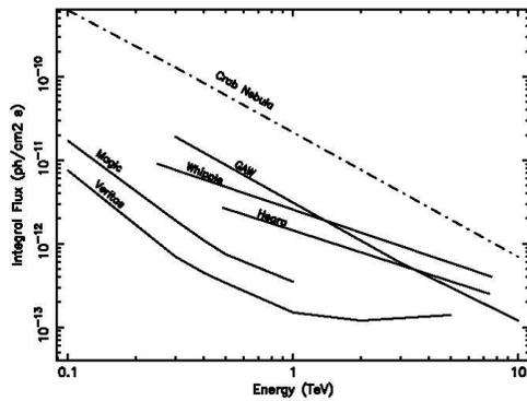
**Fig.2** The sensitivity ( $5\sigma$ ) detection of GAW for point-like sources in 50 hours observations. The sensitivity limit is here evaluated in the case of a Crab-like spectrum during the first phase ( $6^\circ \times 6^\circ$  FoV) of GAW operation.
