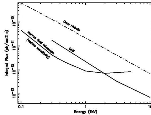
**Fig.3** The capability of GAW to perform deep sky survey with enlarged FoV ( $24^\circ \times 24^\circ$ ). The GAW sensitivity is compared with that reachable in the same time interval by a small field telescope covering the same FoV with many independent pointings.
