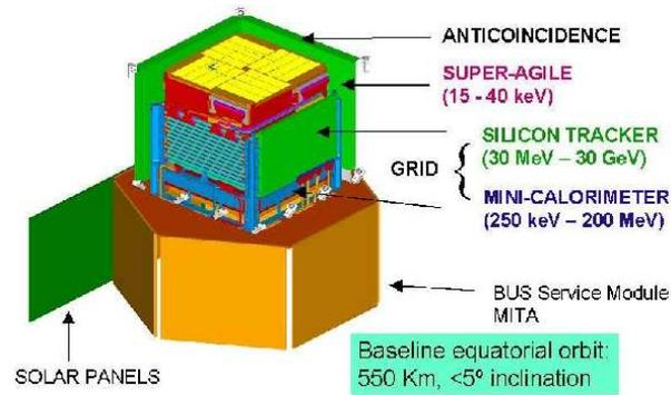
**Fig. 1** The AGILE instrument is light (total payload weight of  $\sim 130$  kg) with a size of  $\sim 63 \times 63 \times 58$  cm<sup>3</sup>.
