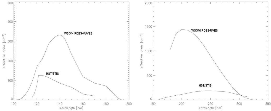
**Fig. 1** A comparison of the effective area of the WSO/UV instruments with that of the UV spectrographs STIS on HST at comparable resolution.
