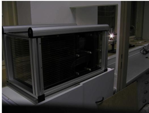
**Fig. 1** The large Lobster Eye telescope prototype ( $300 \times 300$  mm plates, Schmidt arrangement) represents the largest Lobster telescope test module constructed so far.
