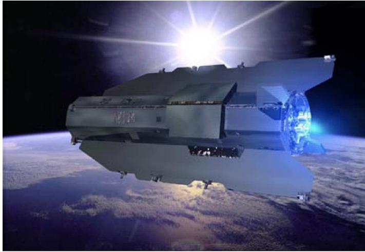
**Fig. 1** The on-going GOCE satellite whose wings allow (at hundred kilometer quota) to gently correct its geodetic for a better and more precise geoid deviations (see Sabatini et al. 2005).
