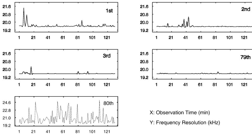
Fig. 7 Changes of frequency resolution at the 1st, 2nd, 3rd, 79th and 80th spectra with observation time.
