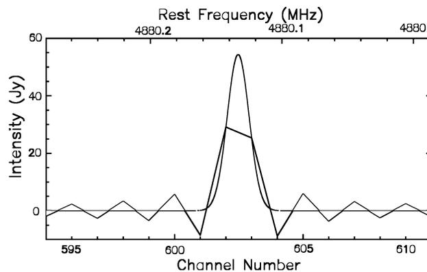
**Fig. 3** A sample spectrum of the response signal of the spectrometer. The black line shows the actual spectrum and the gray line the fitted spectrum.
