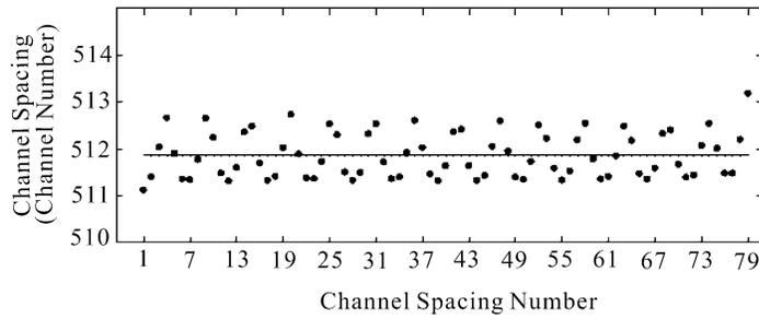
**Fig. 4** Average number of channels covered by each channel spacing. The black dots mark the channel numbers that each channel spacing covers and the straight line marks the theoretical value of 51.18988 channels.
