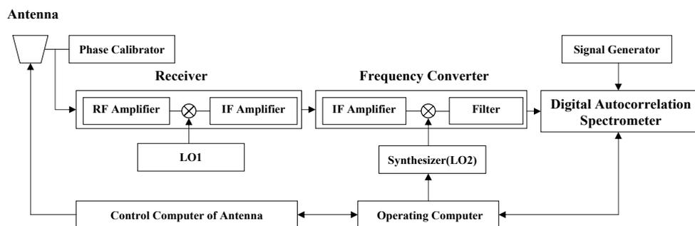
**Fig. 1** Block diagram of the experiment system.
