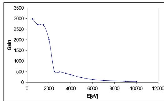
**Fig. 3** The gain, computed from a ray-tracing simulation, as a function of the energy (for one module described in the Figs. above). We define gain as  $g=N1/N2$  where  $N1$  is the number of photons focussed by the LE into area of the size of FWHM (Full Width of Half Maximum) of the PSF (Point Spread Function) and  $N2$  is the number of photons which would be detected in the same area without the focussing power of the LE (Sveda 2003).
